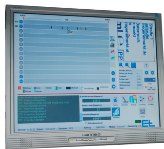
Figure 5: Integration of a Nyscan print image inspection system in a Gallus RCS 330.
