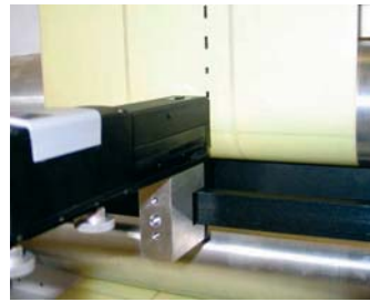
Figure 4: Application of a position code by inkjet printer.
